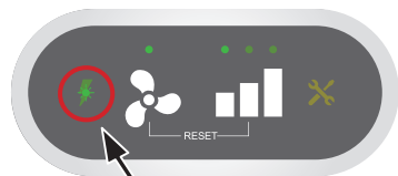
Fixed green LED: the device is on
